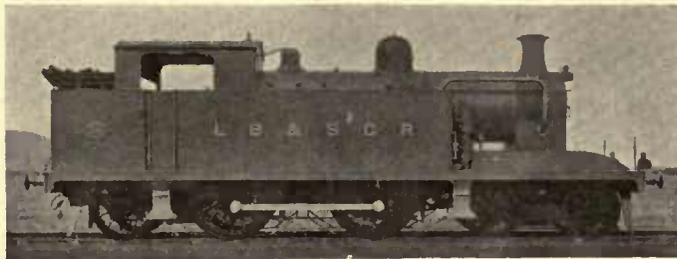
4-4-2 TYPE PASSENGER TANK LOCOMOTIVE L.B. & S.C.R.
