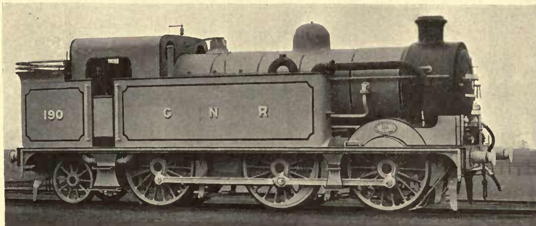
SIX-COUPLED RADIAL (0-6-2 TYPE) TANK LOCOMOTIVE, GREAT NORTHERN RAILWAY.
